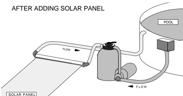
Attach the other end of the 'outlet' hose onto the pool inlet (the place that you removed the first hose from). If you already have another type of heater (like a gas heater) on your pool, plumb in the solar heater upstream (before) the other heater.
