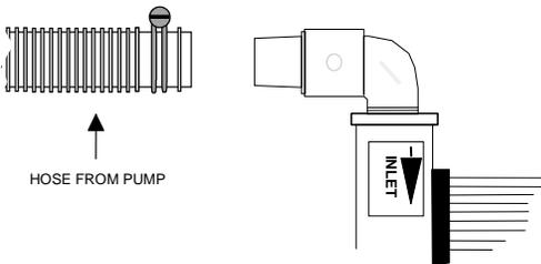
With the clamp in place, push and twist the hose onto the hose barb labeled 'inlet' on your Solar Bear solar heater. Tighten clamp. *NOTE: You may need to warm the end of the hose to make it more pliable. This can be accomplished by placing it in hot water for several seconds.*
