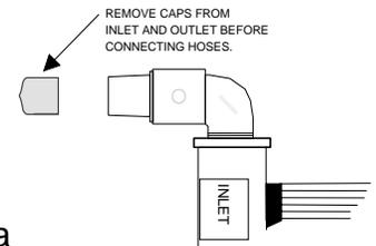
**!** *Remove and discard the caps that cover the inlet and outlet plumbing on your Solar Bear panel. Keep the strap on and the panel rolled up until instructed to unroll it.*
