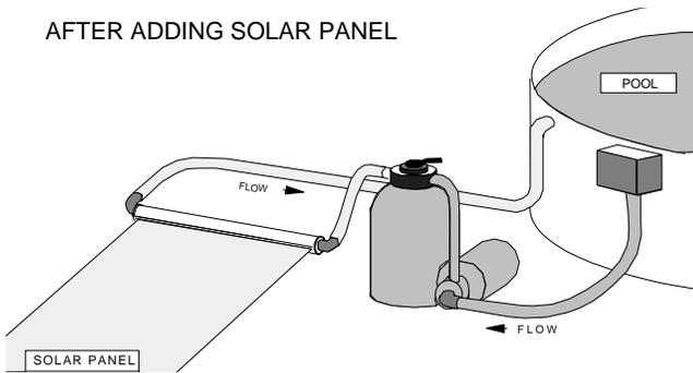
Attach the other end of the 'outlet' hose onto the pool inlet (the place that you removed the first hose from). If you already have another type of heater (like a gas heater) on your pool, plumb in the solar heater upstream (before) the other heater.
