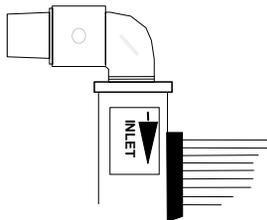
With the clamp in place, push and twist the hose onto the hose barb labeled 'inlet' on your Solar Bear solar heater. Tighten clamp. *NOTE: You may need to warm the end of the hose to make it more pliable. This can be accomplished by placing it in hot water for several seconds.*
